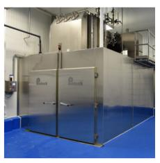
Single door with adjustable solid stainless steel hinges and replaceable silicone door gasket. (Optional: quillotine door.)
