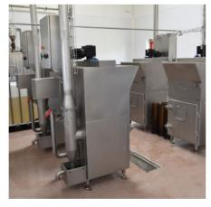
The smoke generator runs on wood chips, sawdust or liquid and creates smoke suitable for all types of products and processes such as cold, hot or steam smoking.
